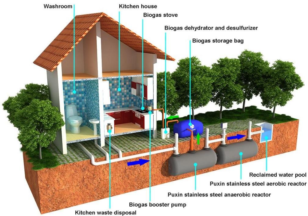
The system is used to process sewage water and food waste as well as small amount of animal waste and is mainly composed of a Puxin stainless steel anaerobic and aerobic reactor, a reclaimed water pool, and the biogas utilization system.
